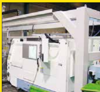
Lathe with digital control
