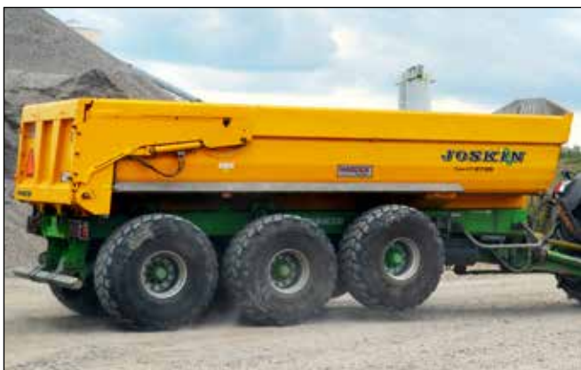
Front lifting axle - standard on Hydro-Tridem
