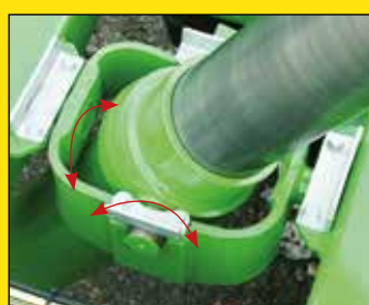
Double oscillating frame in which the ram is placed
